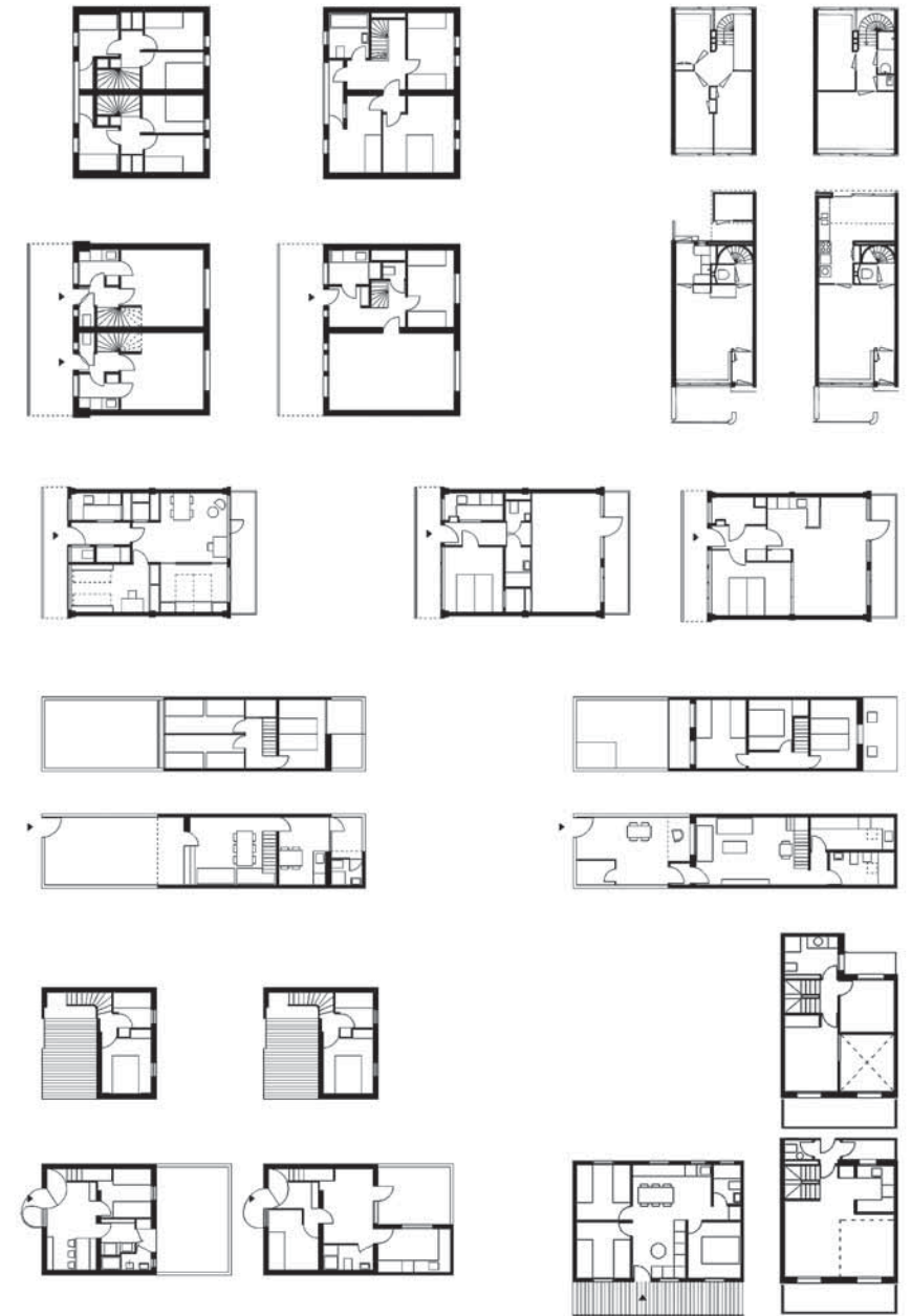
Typical housing unit transformation in the Justus van Effenblok, Kiefhoek and Bergpolder housing buildings (Rotterdam), and the Entrevías, Fuencarral B and UVA Hortaleza housing estates (Madrid). Drawings by Isabel Rodríguez Martín and Sergio Martín Blas.
